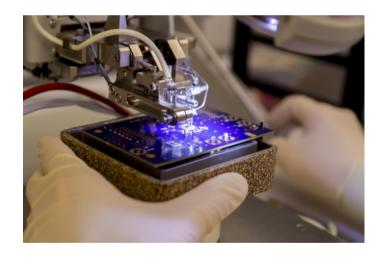
We have leading-edge bonders installed on our manufacturing line from Kulicke & Soffa (K&S) and from Hesse Mechatronics. The newest are the Hesse systems – a Bondjet BJ855 fine wire wedge bonder and a Bondjet BJ939 heavy wire wedge bonder. With our portfolio, we can perform gold, aluminum, copper and silver wirebonding, as well as heavy-wire, wedge and ball bonding, and ribbon bonding.
